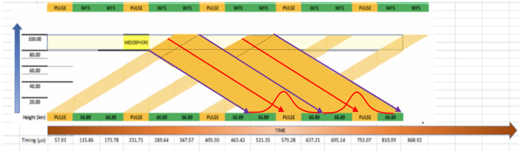
Sketch of the laser pulse duty cycle and the expected measured signal
