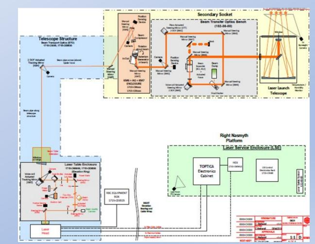
Center launch system to support single laser guide star operations and 4 laser guide star operations for LTAO
